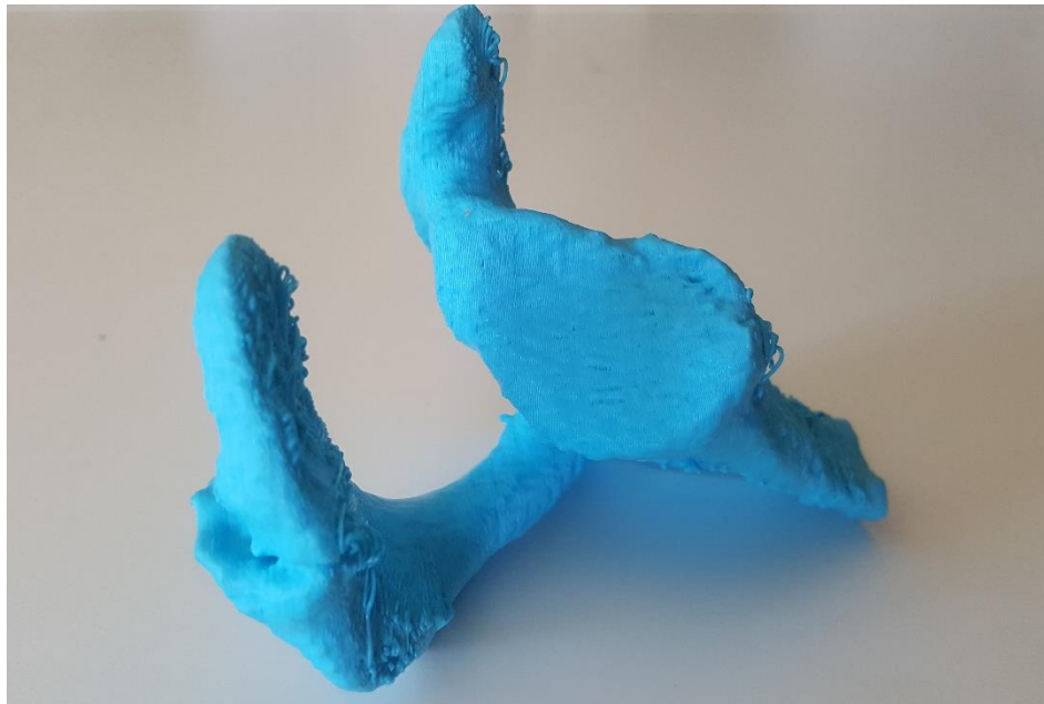
Figure 6. 3D Printed Scapula Model made by PLA (Polylactic acid) material.
