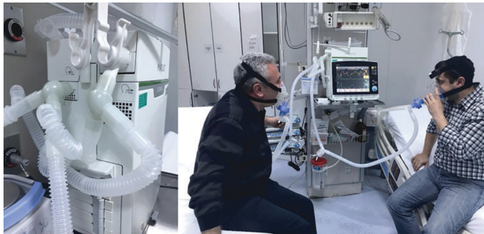
FIG. 3. 3D-printed two-port splitter that adapted both the inspiratory and expiratory outputs of the ventilator and the testing process by two intensive care specialists.
