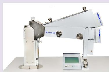
Figure 3. Hecus SWAXS system on our laboratory [7]
